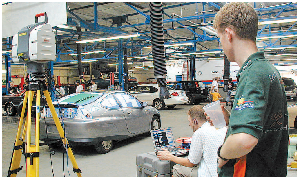
3-D LASER scanning engineers from Boston's Harry R. Feldman Inc.'s land surveying firm spent a day helping the student team at the Vehicle Design Summit at MIT perform six 3-D laser scans of a Honda Insight, pictured above, to make the vehicle more aerodynamic.
