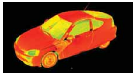
Honda Insight image - scan cloud after all scans were registered.
